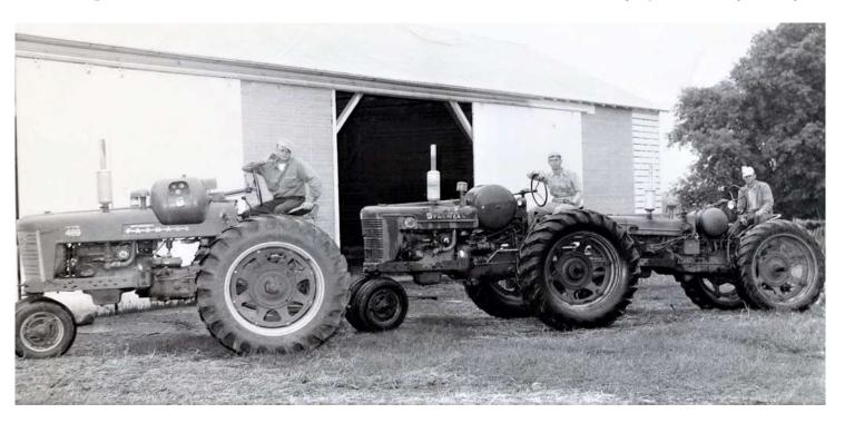
BELOW: This is another Phinney photo from around 1930. This is a Farmall F-20. Notice the two tank setup. No water tank on this tractor. IH engineers have solved the pre-ignition problem with improved engine cooling. The F-20 has a sack of feed riding on the drawbar. Apparently his tractor was handy enough to help with simple chores. In the background: windmill, water pump, barn and grain bin.
