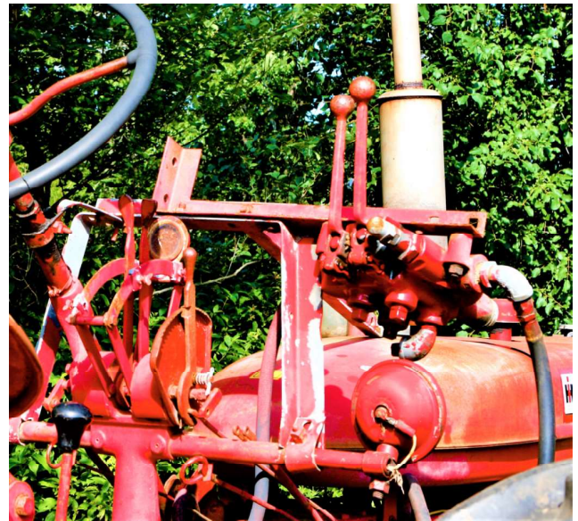
ABOVE: This view of a Farmall Super C shows the remnants of hardware which was added to operate a mounted loader. The two levers just right of the steering column are the factory supplied controls for lifting a cultivator. Everything else, valves, hoses, and a since-removed reservoir tank, was added by a former owner for use with the loader. The angle-iron brackets held the extra two gallon oil tank. Messy, but effective.
