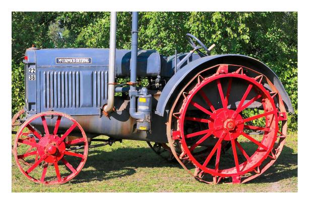
ABOVE and BELOW. These two tractors were both manufactured in the late 1920. They were both built with steel wheels. Rubber tires were widely available by 1937. Sometime after 1937, and probably soon after, the tractor below was converted from steel wheels to rubber tires. That may have been done by the hometown International Harvester dealer or by a local blacksmith.
