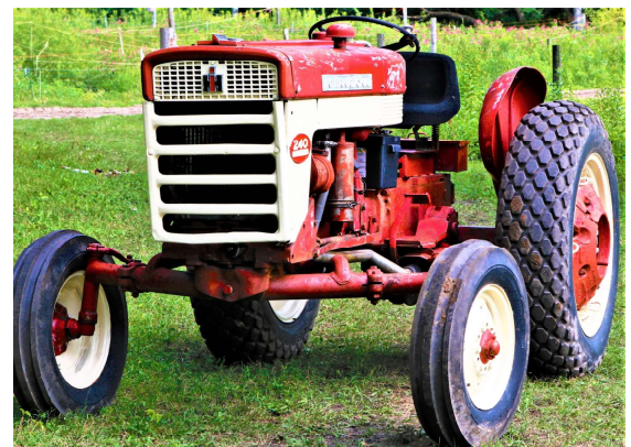
ABOVE: The International 240 Utility is not an original Fairway. Those were specially manufactured row crop tractors. This tractor is what passed for a golf course (fairway) tractor in the 1960s. Note the special turf (grass) tires.
