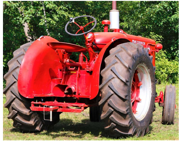
ABOVE: McCormick W-6 Standard. Swinging drawbar, fixed, widely spaced wheels, and semi-closed operator's platform all help to identify a Standard.
