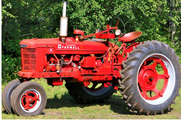
ABOVE: Farmall H row crop. Narrow front, adjustable with rear wheels, high clearance all identify a row-crop.
