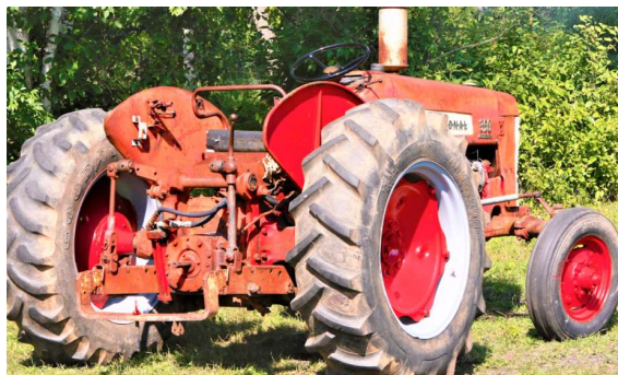
ABOVE: This International 350 is a classic Utility tractor. Low, wide stance, lots of hydraulics, versatile FAST HITCH drawbar, lights and shield fenders.
