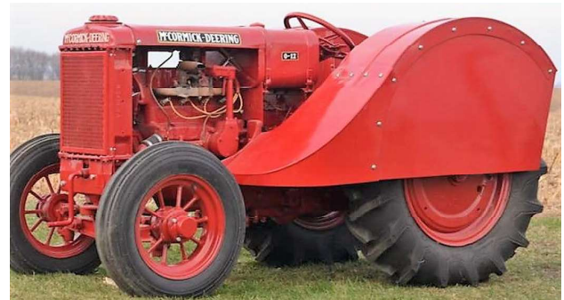
ABOVE: This O-12 Orchard model is easily identified by the sweeping sheet metal and lack of obstructions such as air inlet and muffler.
