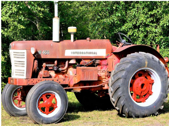
ABOVE: This W 450 Standard that can be further identified as a Wheatland (or Western as you prefer) by the over-the-tire fenders.
